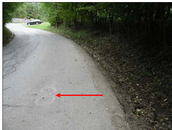
Figure 3: Area of impact viewed from Ford's approach, arrow shows impact gouges in the roadway
