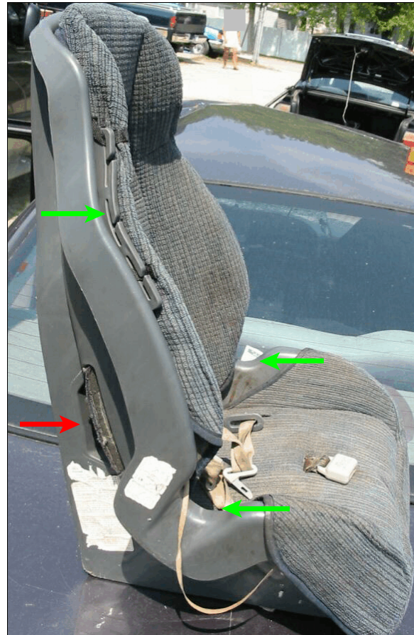
Figure 14: Child safety seat, red arrow shows belt path, green arrows shows shoulder belt slots and lap belt path for use as a belt positioning booster
