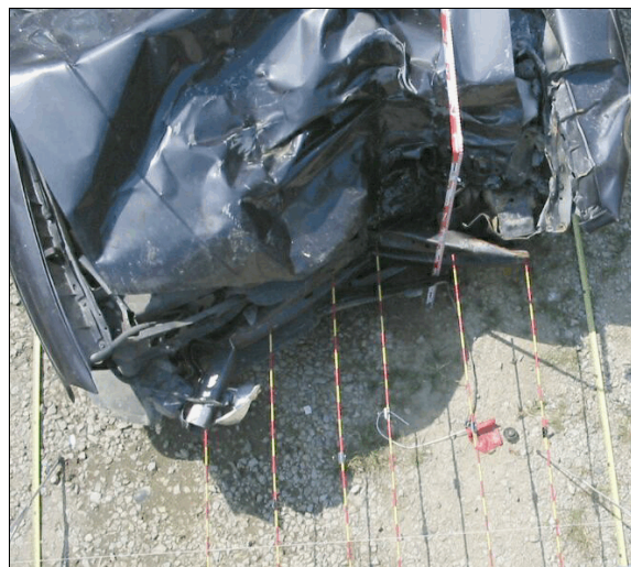
Figure 8: Top view of crush to front of case vehicle
