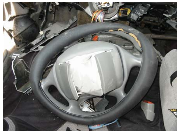
Figure 11: Case vehicle steering wheel deformation and air bag module cover flaps
