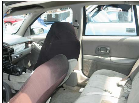
Figure 10: Overview of case vehicle's back right seat position and deformation of front right seat back
