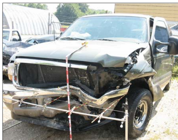
Figure 5: Overview of damage to front of Ford from impact with front of case vehicle
