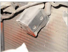
Figure 8: Close view of case vehicle's left discriminating sensor, crushed rearward into radiator condenser
