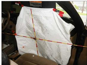
**Figure 13:** Overview of case vehicle's deployed front right passenger air bag
