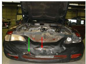
Figure 6: Front of case vehicle with vinyl skirt in place, green arrow shows cut from contact with Windstar's tail pipe, red arrow shows tear in vinyl from contact with bottom portion of Windstars back bumper
