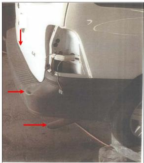
**Figure 5:** Attorney provided photo of right side view of damage to back of Windstar (arrows) from impact with case vehicle, right tail lamp assembly has been removed
