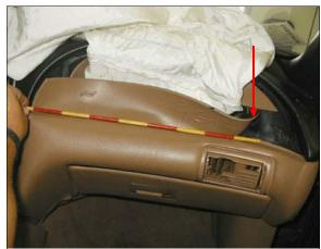
**Figure 12:** Case vehicle's front right passenger's air bag module cover flaps, arrow shows deformation of lower cover flap
