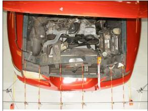
Figure 10: Top view of crush to top radiator support
