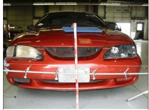
Figure 3: Damage to front of case vehicle from impact with back of Windstar
