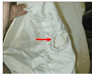
**Figure 14:** Case vehicle's front right passenger air bag vent port (arrow)
