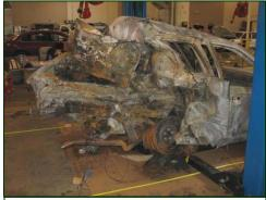
Figure 6. Right side view of the extent of crush and deformation.
