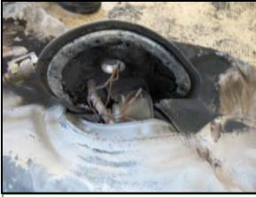
Figure 18. Displaced sending unit from forward aspect of tank.
