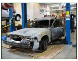
Figure 8. Front left view of the CVPI and associated fire and rescue damage.
