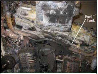
Figure 15: Deformed undercarriage of subject CVPI.
