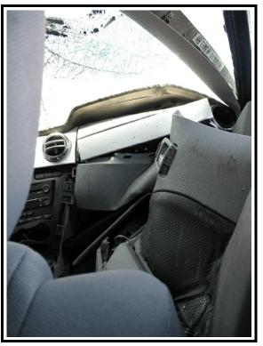
**Figure 16**. Front right seat position, shows lateral door intrusion
