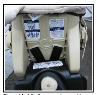
Figure 12. Misalignment of seat and base
