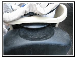
Figure 10. Base release lever
