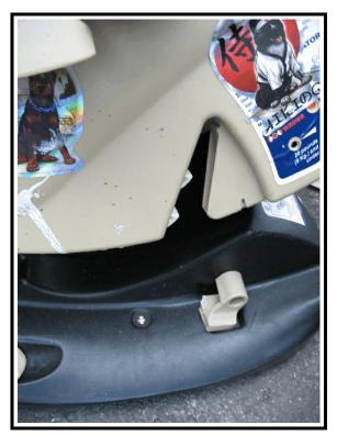
**Figure 13**. Child seat and base attachment point
