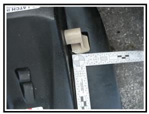
Figure 11. Damage to base attachment
