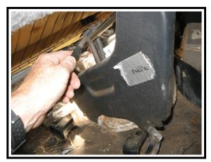
**Figure 15**. Seat locking lever, third row right
