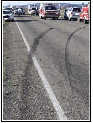
**Figure 5**. Left front and left rear tires approaching trip point
