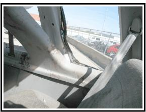
**Figure 31**. Contact to D pillar from Occupant 12.
