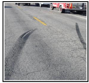
**Figure 6**. Left front and left rear tires at trip point–left rear gouging roadway
