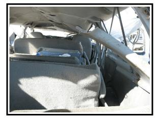
Figure 13. Overview of intrusion, left side
