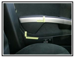
**Figure 18.** Possible occupant contact points to the LF door panel and armrest (2006 Nissan Maxima)
