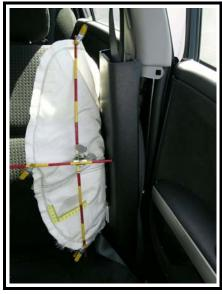
**Figure 8**. Intrusion of the B pillar cover and scuff to the deployed outer driver side air bag
