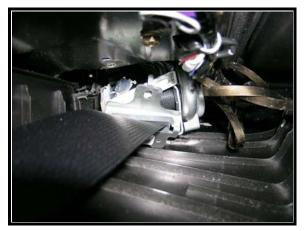
**Figure 10.** Damaged LF seat belt retractor (2006 Nissan Maxima)
