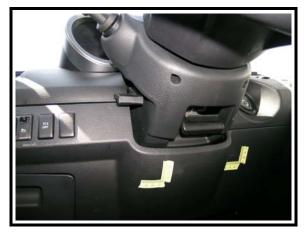
**Figure 17**. Possible driver contacts below steering column (2006 Nissan Maxima)
