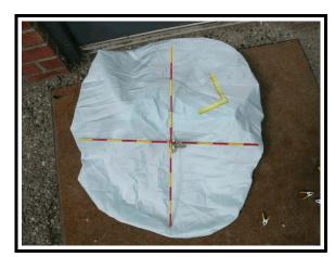
**Figure 16**. Front right passenger air bag - 2000 Honda Odyssey (removed during repair)
