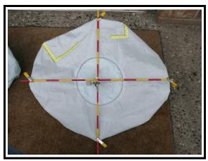
**Figure 15**. Driver air bag - 2000 Honda Odyssey (removed during repair)
