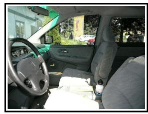
**Figure 14.** RF seat and possible occupant contact to the RF door panel (2000 Honda Odyssey)
