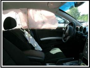
**Figure 12**. Deployed left side curtain (2006 Nissan Maxima)
