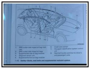
**Figure 11.** Supplemental Safety System & Sensor Locations (2006 Nissan Maxima)
