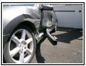
**Figure 7**. Bumper of the 2000 Honda Odyssey still embedded in the left front door (2006 Nissan Maxima)
