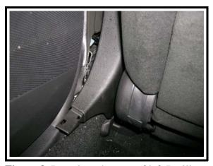
**Figure 9**. Intrusion - bottom of left B pillar cover. The RFBC of the Honda Odyssey intruded through the Maxima's LF door panel.
