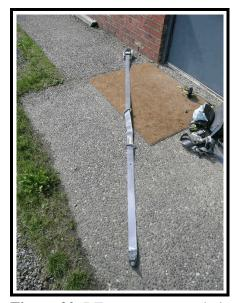
**Figure 20**. RF passenger seat belt - removed during repair (2000 Honda Odyssey)
