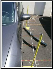
**Figure 6**. Crush profile - 2006 Nissan Maxima
