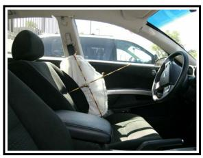
**Figure 13**. Deployed driver side air bag (2006 Nissan Maxima)
