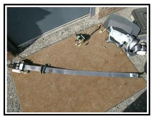
**Figure 19**. Driver's seat belt - removed during repair (2000 Honda Odyssey)
