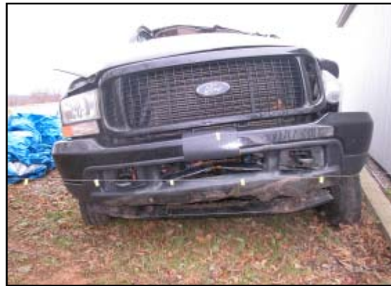
Figure 4. Frontal damage from the delineator post.
