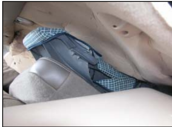
Figure 10. Damage to the right side of the belt positioning booster seat.
