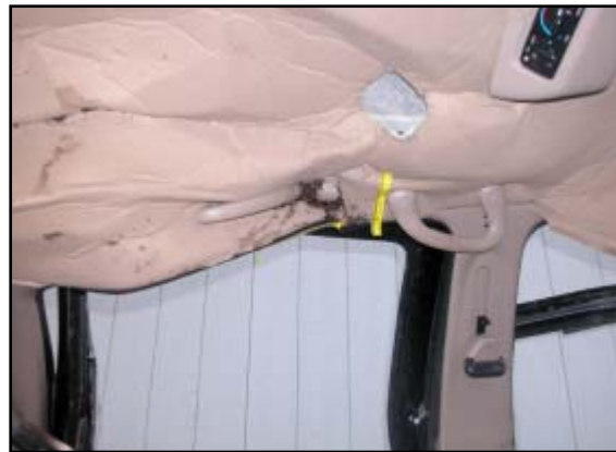
Figure 8. Left roof side rail denting/pocketing and body fluid.
