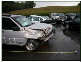
Figure 8. Frontal crush to the Cherokee.
