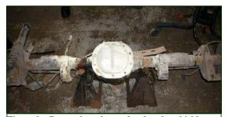
Figure 9. Rear axle and sway bar bracket shields.
