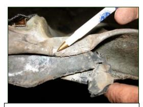
Figure 11. Strap puncture of fuel tank.
