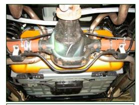
Figure 15. Exemplar CVPI with FirePanel installed.
