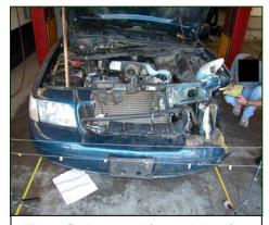
Figure 5- Damaged front plane of 2003 CVPI.
