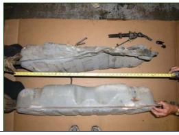
Figure 13. Damaged and exemplar fuel tanks.
