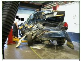
Figure 3. Damaged back plane of 2003 Ford CVPI.
