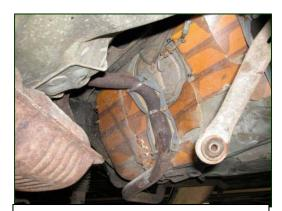
Figure 16. Damaged FirePanel.
