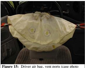
**Figure 15:** Driver air bag, vent ports (case photo #73)
