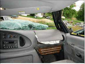
**Figure 17:** Overview of front right instrument panel and air bag location (case photo #81)
