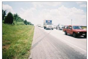
**Figure 2:** On-scene photo showing four tire marks from the case vehicle on shoulder; tire marks are (from bottom to top): left rear, right rear, left front and right front (case photo #150)
