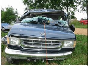
**Figure 7:** Crush of right A-pillar and roof; each stripe on the rod is five centimeters (two inches), (case photo #34)
