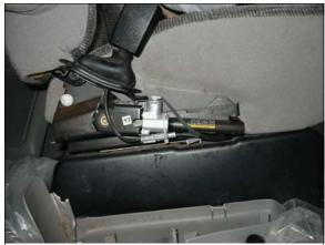
Figure 19: Driver's safety belt pretensioner did not activate; the buckle stalk is not shortened and the stalk cover is not compressed (case photo #67)
