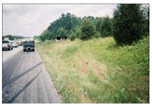
Figure 3: On-scene photo showing tire marks on shoulder and ground; marks are (from left to right): left rear, right rear, left rear ground divot, left front ground divot, right front ground divot (case photo #150)
