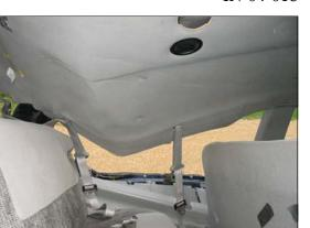
Figure 11: Roof and roof side rail intrusion into the third back seat row (case photo #129)
