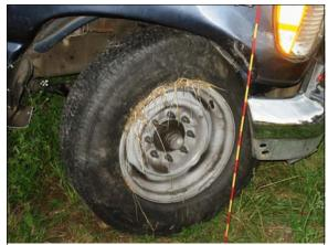
Figure 8: Right front wheel inflated and restricted by damage (case photo #50)
