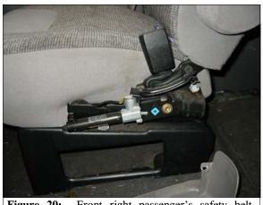
**Figure 20:** Front right passenger's safety belt pretensioner activated; the buckle stalk is shortened and the stalk cover compressed (case photo #90)
