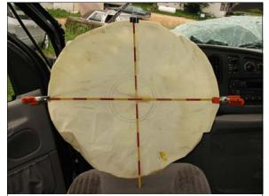
Figure 14: Driver's air bag; each stripe on rod is five centimeters (two inches), (case photo #71)
