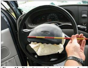
Figure 13: Driver's top air bag module cover flap (case photo #75)
