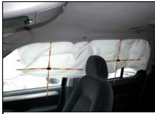
Figure 15. Deployed right side safety canopy air bag.
