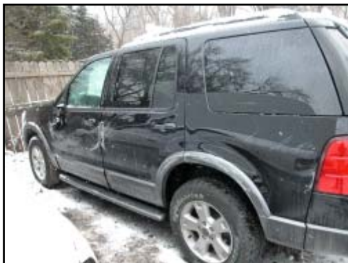
Figure 9. Rollover damage to the left side of the Ford.
