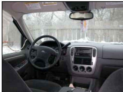
Figure 16. Ford's instrument panel, no frontal air bag deployment.
