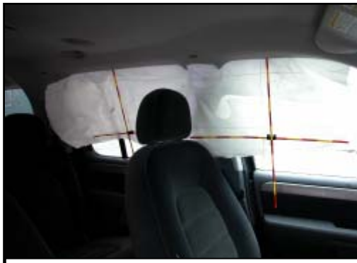
Figure 14. Deployed left side safety canopy air bag.
