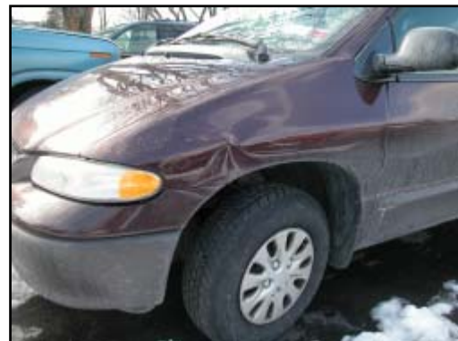
Figure 13. Damage sustained from the impact with the Ford.
