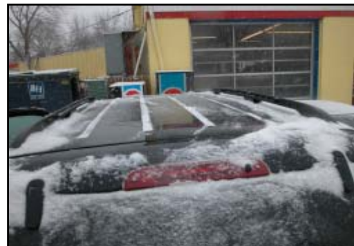
Figure 10. Rear roof aspect of the Explorer. Note no damage from the impact with the Dodge.
