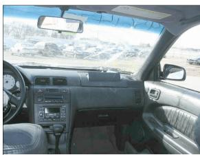
Figure 16: Case vehicle's front right passenger seating area showing deployed front right passenger air bag, stress cracks to windshield's glazing, and no apparent evidence of occupant contact to interior surface of right front door, right instrument panel, or greenhouse areas (case photo #36)
