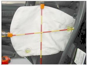
**Figure 24:** Outboard side of case vehicle's deployed driver side impact air bag (case photo #55)
