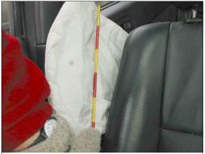
**Figure 27:** Inboard side of case vehicle's deployed right front side impact air bag (case photo #52)
