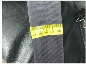
Figure 29: Lap belt portion of case vehicle's driver safety belt showing loading mark from latch plate (case photo #60)
