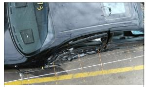
Figure 14: Overhead view of case vehicle's right side damage showing crush positions 1 through 5 (case photo #30)
