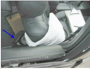
Figure 22: Overhead view of case vehicle's deployed right front side impact air bag; Note: arrow shows bag's cover flap (case photo #50)
