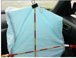
Figure 21: Close-up of scuff (highlighted) on case vehicle's deployed front right passenger air bag (case photo #45)
