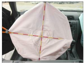
Figure 19: Case vehicle's deployed driver air bag showing no apparent evidence of occupant contact (case photo #40)
