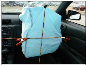
Figure 20: Front surface of case vehicle's deployed front right passenger air bag showing only a small area (i.e., scuff) of occupant contact near the 12 o'clock position (case photo #44)
