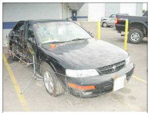
Figure 8: Case vehicle's right side damage viewed from right of front; Note: damage rearward of right "A"-pillar (case photo #27)
