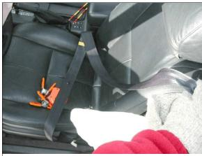
**Figure 28:** Loading evidence on lap portion of case vehicle's driver safety belt (case photo #59)
