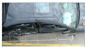
Figure 13: Overhead view of case vehicle's right side damage showing crush positions 2 through 6 (case photo #29)
