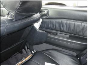
Figure 23: Case vehicle's front right seat back showing cover flap for right front side impact air bag (case photo #54)
