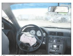
Figure 15: Case vehicle's driver seating area showing deployed driver air bag, stress cracks to windshield's glazing, and no obvious occupant contact evidence (case photo #34)
