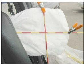
**Figure 25:** Inboard side of case vehicle's deployed driver side impact air bag (case photo #56)
