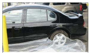
Figure 9: Left side view of case vehicle's undamaged left side except for bead separation to and deflation of left rear wheel (case photo #19)
