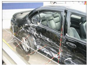
**Figure 12:** Case vehicle's right side damage with contour gauge positioned above sill showing crush at 1<sup>st</sup> through 4<sup>th</sup> positions (case photo #24)
