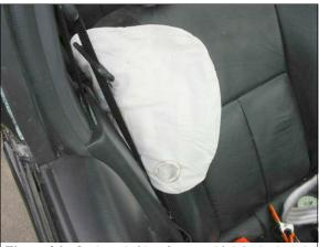
**Figure 26:** Outboard side of case vehicle's deployed right front side impact air bag (case photo #51)
