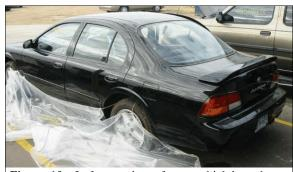
**Figure 10:** Left rear view of case vehicle's undamaged left side except for bead separation to and deflation of left rear wheel (case photo #20)
