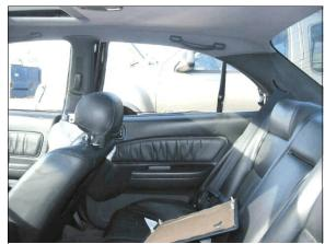
**Figure 18:** Interior surface of case vehicle's right rear door showing 16 cm (6.3 in) of intrusion to back right seating area (case photo #64)
