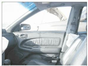
Figure 17: Interior surface of case vehicle's right front door showing no obvious occupant contact evidence on intruding surface (case photo #31)
