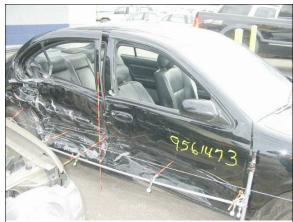
**Figure 11:** Case vehicle's right side damage with contour gauge positioned above sill showing crush at 2<sup>nd</sup> through 6<sup>th</sup> positions (case photo #25)
