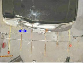
Figure 7: Overhead view of case vehicle's frontal damage with contour gauge present at bumper level; arrow indicates location of pole impact (case photo #22)
