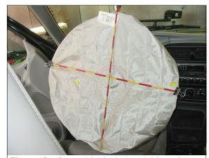
**Figure 13:** Case vehicle's deployed driver air bag showing (i.e., yellow tape) blood spots near 3 o'clock position and between center and 9 o'clock position (case photo #27)
