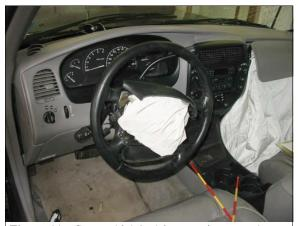
Figure 11: Case vehicle's driver seating area showing deployed frontal air bags, driver's toe pan area, and left instrument panel; Note: no obvious contact evidence present (case photo #26)
