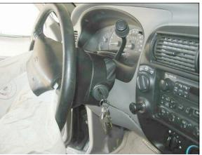
Figure 8: Case vehicle's slightly deformed steering wheel rim and loaded steering column; Note: steering column driven forward against left instrument panel (case photo #38)
