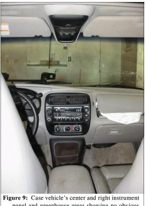
Figure 9: Case vehicle's center and right instrument panel and greenhouse areas showing no obvious evidence of occupant contact and crack to right windshield's glazing (case photo #40)
