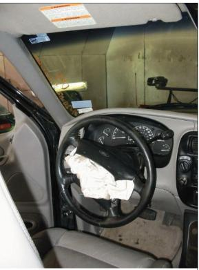
Figure 10: Case vehicle's driver seating area showing deployed driver air bag and no obvious contact evidence to greenhouse area or right side of driver's knee bolster (case photo #25)
