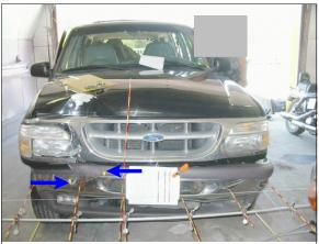
Figure 4: Case vehicle's frontal damage with contour gauge set at bumper level; Note: yellow tape (arrows) shows location and direct damage width of pole impact (case photo #10)
