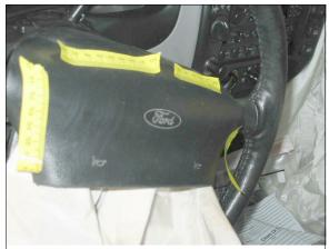
Figure 12: Vertically oriented scuffs on case vehicle driver air bag module's top cover flap (case photo #34)
