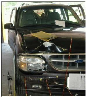
Figure 6: Case vehicle's front right damage from impact with utility pole viewed along right side (case photo #21)
