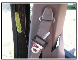
Figure 22. Possible contact to C pillar/side glass frame
