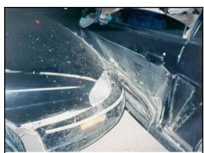
Figure 2: Case vehicle's front against other vehicle's left side at final rest, showing case vehicle's right front corner area (case photo #19)
