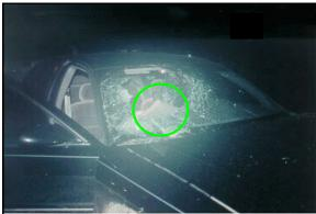
**Figure 4:** Case vehicle at final rest; note, large hole in windshield with passenger air bag module cover flap projecting through (case photo #07)
