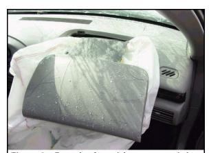
**Figure 6:** Exemplar front right passenger air bag cover flap, showing tethered installation NOT THE CASE VEHICLE (case photo #28)
