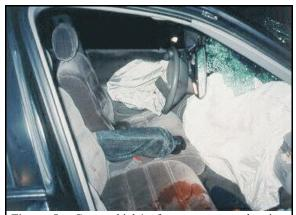
Figure 5: Case vehicle's front seat row, showing deployed air bags, fractured windshield and blood on the front right seat cushion (case photo #08)
