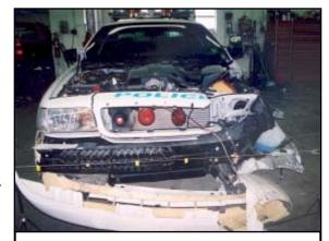
Figure 3. Resultant frontal damage to the Ford.
