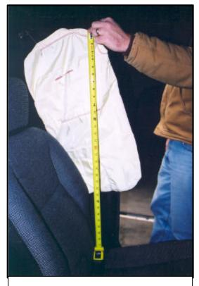
Figure 8: Deployed side impact air bag.
