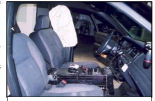
Figure 7: Right interior view depicting the deployed side impact air bag.
