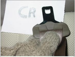
Figure 24: Latch plate for case vehicle's second seat center position showing no obvious evidence of loading (case photo #60)
