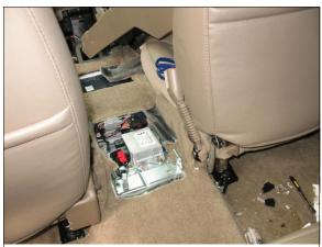
Figure 22: Case vehicle's Restraints Control Module which was located under the floor, below the center console, and between the front bucket seatsviewed from second seating area (case photo #48)
