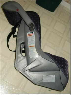
**Figure 21:** Case vehicle's Century convertible child safety seat laid on its left side in forward facing configuration showing tray shield, top tether, and warning labels (case photo #65)
