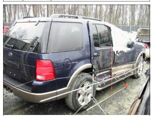
Figure 5: Case vehicle's right side damage viewed from right of back with contour gauge present (case photo #23)
