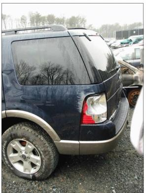
Figure 12: Rollover damage to case vehicle's left quarter panel and tail/brake/stop light assembly (case photo #20)
