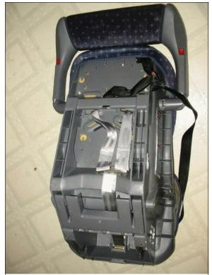
Figure 20: Back surface of Century convertible child safety seat used by case vehicle's second seat center passenger showing tray shield, top tether, and no apparent evidence of damage to back surface (case photo #70)
