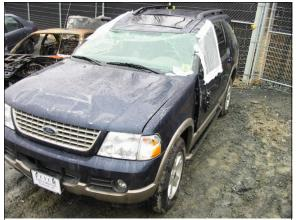
Figure 7: Elevated view from left of front showing rollover damage to case vehicle's hood, roof, and left front door areas (case photo #19)
