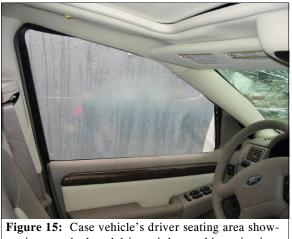
ing non-deployed driver air bag and intrusion into occupant's space from roof, roof side rail, left "A"-pillar, and windshield (case photo #33)
