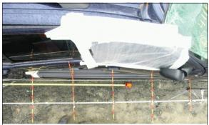
Figure 11: Overhead view of case vehicle's left side damage showing crush with contour gauge present (case photo #27)
