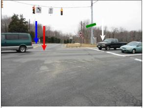
Figure 8: Westward view of crash scene showing approximate point of impact (red arrow), case vehicle's approximate final rest position on roof (blue arrow), and Chevrolet's (white arrow) converging trajectory (case photo #04)
