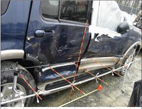
Figure 9: Closer-in view of case vehicle's right side damage with contour gauge present (case photo #24)
