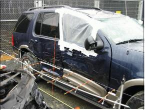
Figure 10: Case vehicle's right side damage viewed from left of front with contour gauge present (case photo #25)
