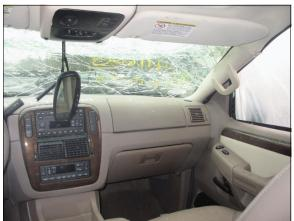
Figure 14: Case vehicle's front right seating area showing non-deployed front right air bag, dislodged rearview mirror, right "A"-pillar and door intrusions, and no occupant contact evidence (case photo #36)
