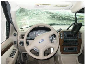
Figure 13: Case vehicle's driver seating area showing non-deployed driver air bag, roof and left "A"-pillar intrusions, and no apparent evidence of occupant contact (case photo #34)
