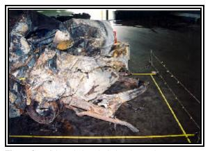
**Figure 8**: Left lateral view depicting the maximum deformation.
