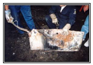
**Figure 14**: Filler neck and fuel tank after removal from the vehicle.
