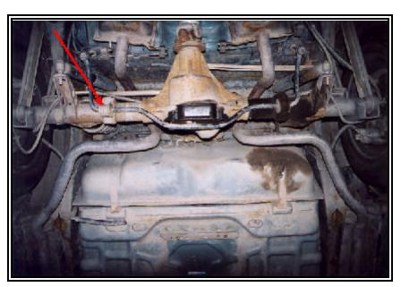
Figure 12: View of the fuel tank and rear axle components of an exemplar Ford Crown Victoria.
