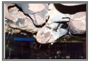
Figure 4: Drive shaft deformation.
