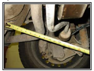
Figure 13: Distance between sway bar bracket and the fuel tank.
