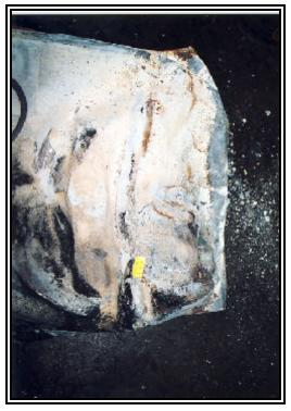
**Figure 17**: View depicting the location of the puncture/cut on the left side of the tank.
