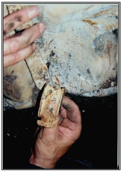
Figure 19: View of the contact between the tank, carry strap and left rear sway bar bracket.
