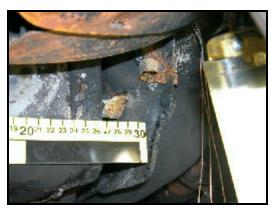
**Figure 9**. Shows wrecking bar exiting trunk (left) and penetrating back of fuel tank (right).
