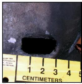
**Figure 10**. Close up of puncture to back of fuel tank(entry)
