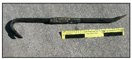
Figure 12. Wrecking bar
