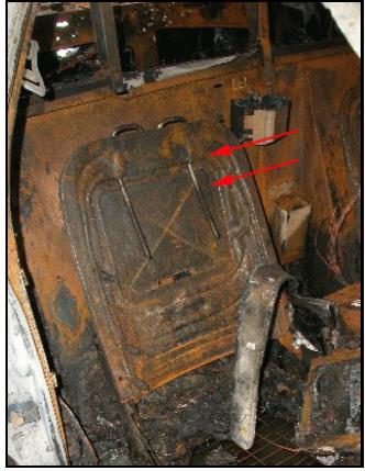
**Figure 19**. Front right seat–head restraint was in up position during the fire
