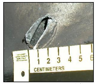
**Figure 11**. Puncture to front of fuel tank (exit)
