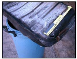
Figure 8. Puncture to back of fuel tank
