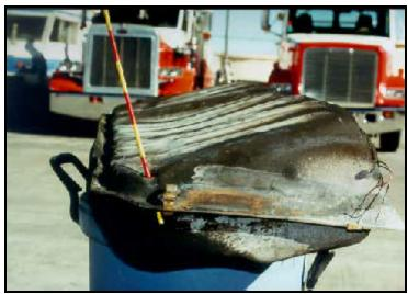
**Figure 14**. Side view of fuel tank showing entry and exit points
