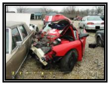
Figure 20. Frontal damage to the Mitsubishi Eclipse
