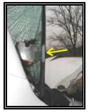
Figure 5. Close-up view of silicone caulk bead on the right aspect of the windshield
