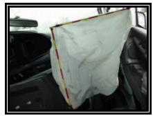
Figure 26. Redesigned front right passenger's air bag
