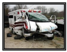
Figure 1. Damaged Type III ambulance
