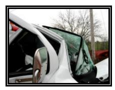
Figure 14. Right side view of windshield bond separation
