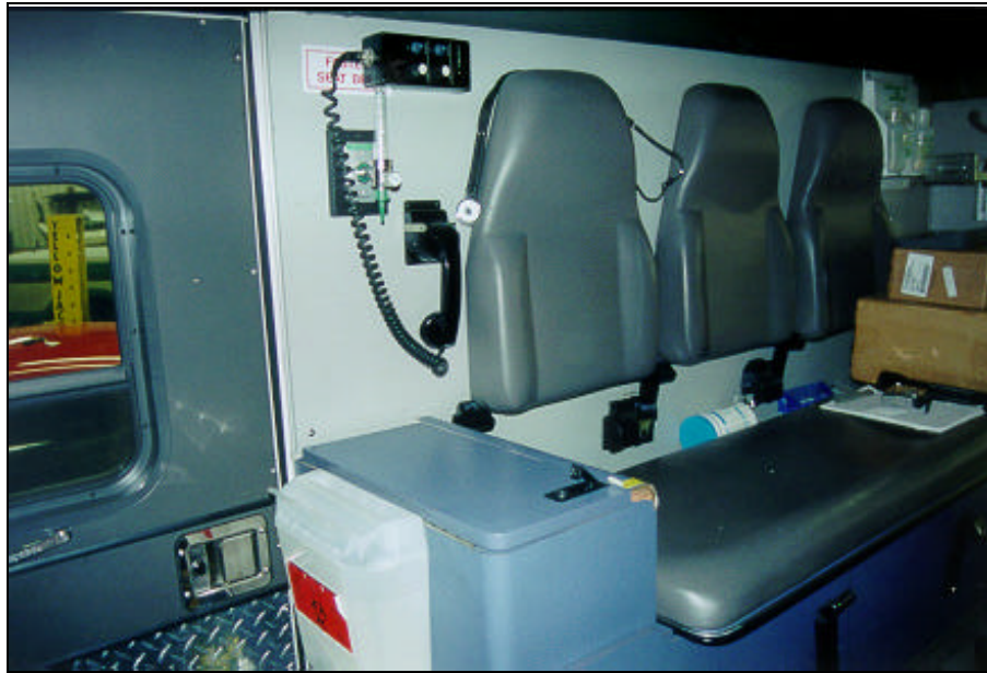
Figure 12. Right side, ambulance compartment—showing squad bench
