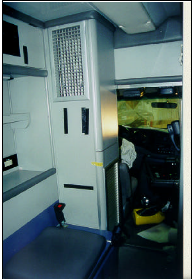
Figure 17. Possible contact to door portal—panel shifted
