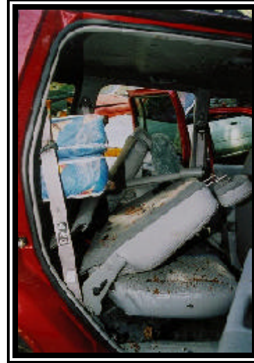
Figure 8. Second row seat back deformation from cargo movement within the vehicle.
