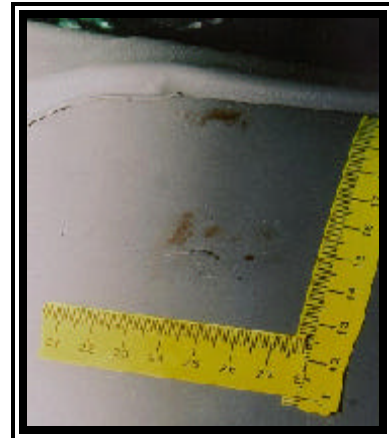
Figure 9. Contact evidence to the non-deployed front right passenger air bag module cover flap.
