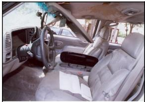
Figure 3: Case vehicle's front seat row, showing collapsed overhead console and right roof rail intrusion from rollover (case photo #25)
