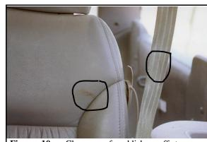
**Figure 10:** Close-up of reddish scuff to case vehicle's third seat left passenger 's seat back and seat belt webbing (highlighted) (case photo #35)
