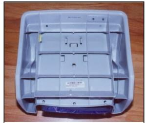
**Figure 9:** Underside view of booster seat showing no visible stress evidence (case photo #39)
