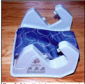
**Figure 8:** Belt-positioning booster seat in use at the time of the crash (case photo #37)
