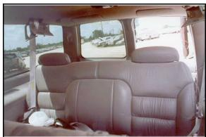
Figure 7: Third seat row; NOTE: seat belt retractor housing hanging out from roof (case photo #32)
