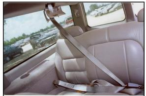
**Figure 11:** View of case vehicle's third row right seat position showing collapsed retractor housing and belt extended (case photo #33)
