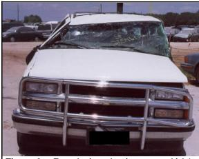
**Figure 6:** Frontal view showing case vehicle's rollover damage (case photo #06)
