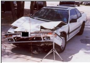
**Figure 12:** Front left view of front end damage to Honda from impacting case vehicle and guardrail (case photo #47)
