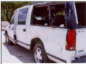
**Figure 5:** View from left rear showing case vehicle's left side damage from impact with guardrail (case photo #12)
