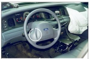
Figure 7: On-scene view of case vehicle's asymmetrical air bag deployment; Note: separation (highlighted) between steering wheel hub and air bag module (case photo #44)
