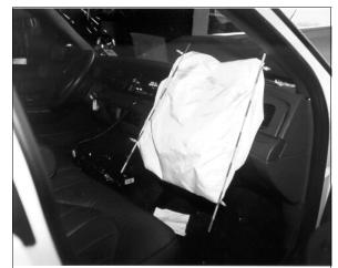
**Figure 8:** Case vehicle's deployed front right passenger air bag showing no evidence of driver contact (case photo #35)
