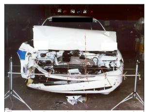
Figure 4: Case vehicle's frontal damage with contour gauge in place for above bumper measurements (case photo #07)
