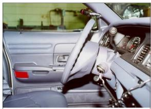
Figure 6: Side view of case vehicle's deformed steering wheel rim; Note: shear capsule movement also occurred (case photo #29)
