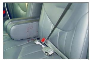
**Figure 9:** On-scene view of case vehicle's buckled, driver seat belt, which was behind driver's back; Note: blood on center arm rest (case photo #45)
