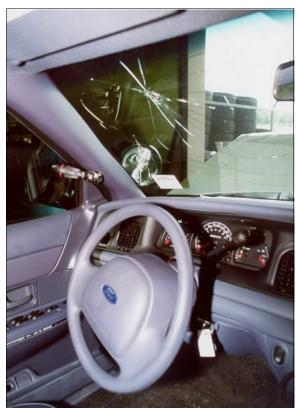
Figure 10: Vertical view of case vehicle's driver seating area showing contacted steering wheel rim, non-deployed driver's air bag, and "spider web" crack on windshield from driver's head contact (case photo #30)
