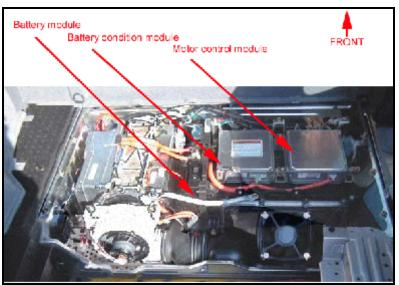
Figure 6. Exemplar view, rear battery compartment. Shows IMA components
