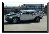
Figure 1. Rollover damage to the 2000 Ford Explorer.
