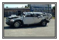
Figure 9. Left side rollover damage to the Explorer.
