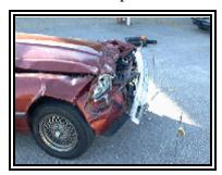
Figure 13. Profile view documenting the extent of frontal crush.
