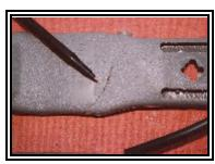
Figure 21. Cut line on the passenger's buckle sleeve.
