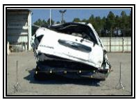
Figure 7. Rear impact damage to the Ford Explorer.
