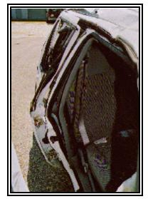
Figure 17. Post-crash position of the retracted right front belt system.
