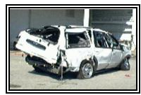
Figure 8. Right threequarter view of the rear damage.
