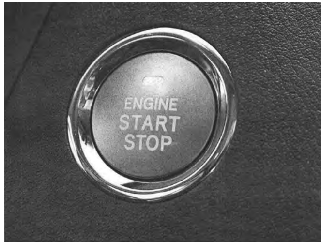
Figure 6—Push Button Ignition Replaces Conventional Key
