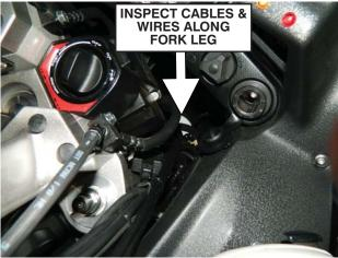
Remove the cable clamp and bracket from the left and right lower-outside triple clamps.
