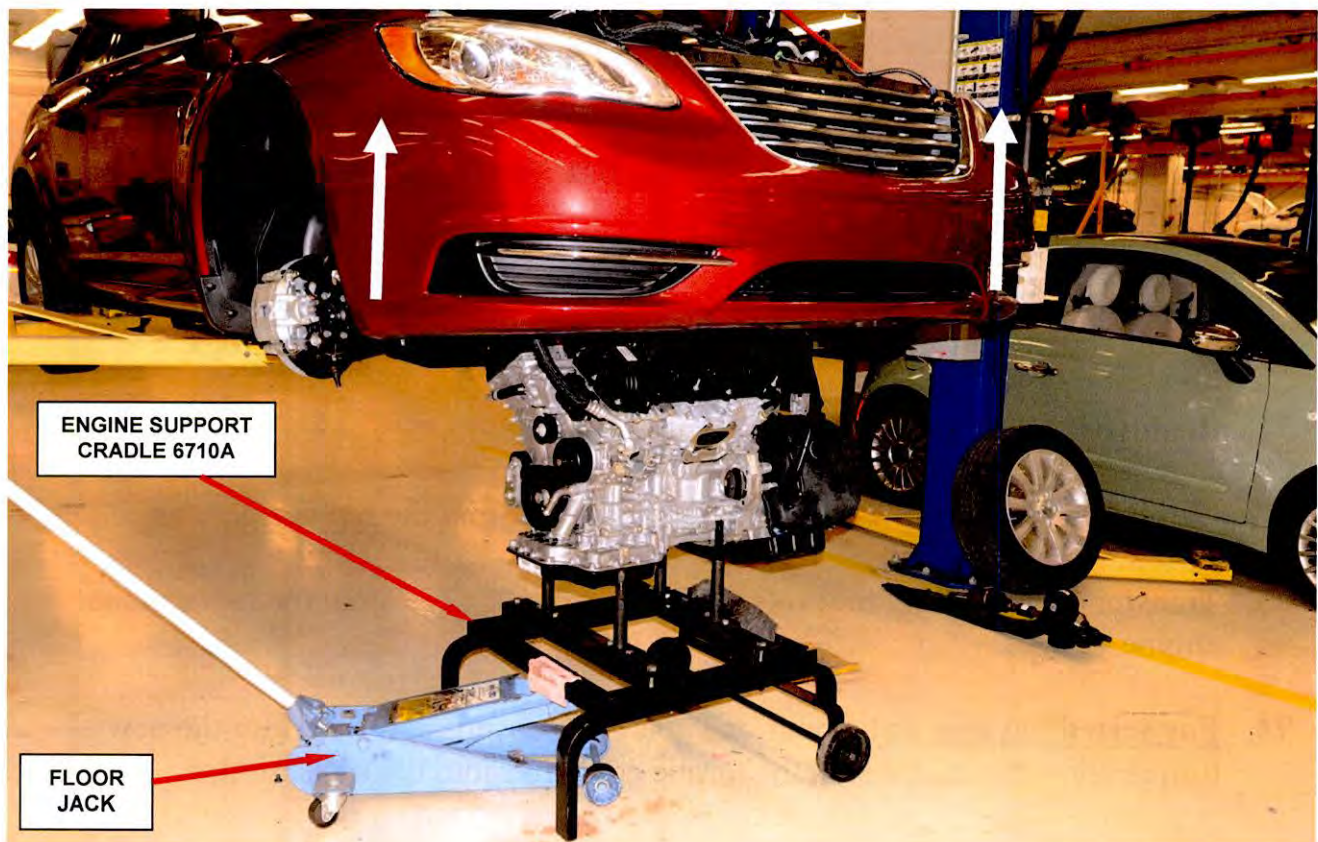
Figure 19 – Guide Engine During Removal
