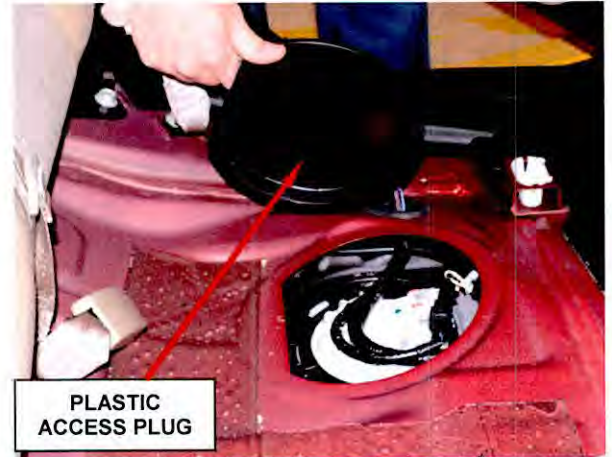
Figure 1 – JS Fuel Pump Access
