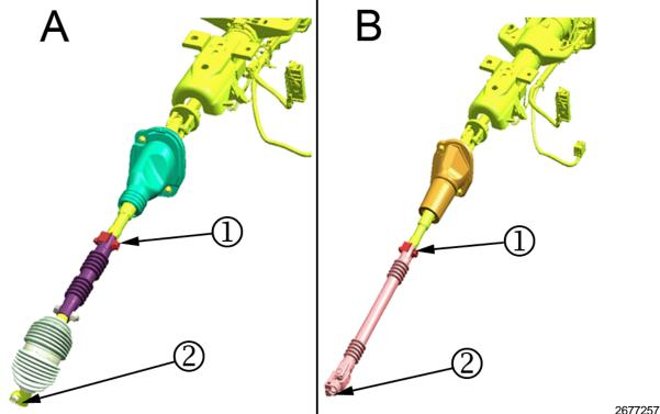
The "A" portion of the illustration provides an example of an intermediate shaft on a 1500 series vehicle. (1) Mid Joint Bolt (2) Pinion Bolt. The "B" portion of the illustration provides an example of an intermediate shaft on a 2500 or 3500 series vehicle. (1) Mid Joint Bolt (2) Pinion Bolt. Hybrid vehicle intermediate shafts are similar to the intermediate shafts in 1500 series vehicles.
