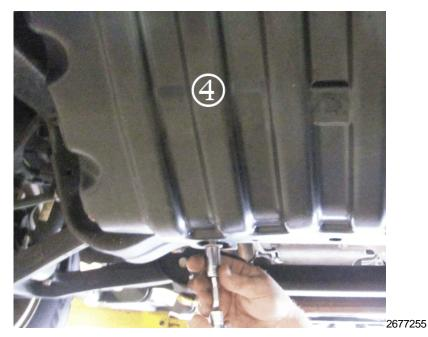
4. Remove the engine shield (4). Refer to Engine Shield Replacement in SI.
