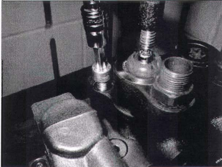
Figure 13 – High Pressure Fuel Pump Element Installation
