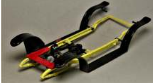
Chassis sub-assembly with engine/transmission installed
