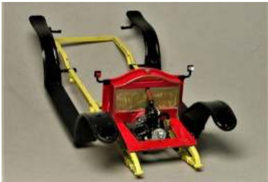
Chassis Sub-assembly with radiator installed
