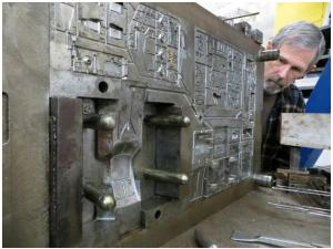
Gerry Humbert examines a mold for a Revell car. The areas for the car's seats, grille and roof are visible in the foreground. The steel support rods keep the steel mold for warping as plastic explodes into the channels at 2,000 lbs. per square inch—roughly the pressure a submarine would experience 4,000' under water, or the weight of 400 compact cars
