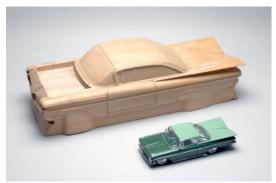
A wooden pattern model of a 1959 Chevy Impala, meticulously carved from basswood. These pattern models, about 2-3 times the size of the finished model, must contain every single detail that is going to be reproduced in plastic—from the dashboard dials to the pattern on the headlight glass.
