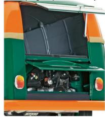
The engine sits in the rear under the back section of the interior floorboard. Any detail work will be visible due to the opening rear door.
