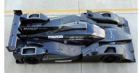
Mazda's oil burners will be carried in the back of P2 chassis built by Canada's Multimatic, which took over production of Lola when the storied British constructor was liquidated. Targets for horsepower and torgue fall in the 450-500 range.
