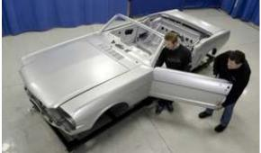
The shell is built with modern welding techniques and comes rustproofed and ready for paint. Ford says suppliers of restoration parts must meet or exceed fit, finish and quality of original. That's why the Mustang body shell is constructed of higher-grade steel than the original, according to Ford. The company allows suppliers to work off old technical drawings, blueprints and specifications for parts.
