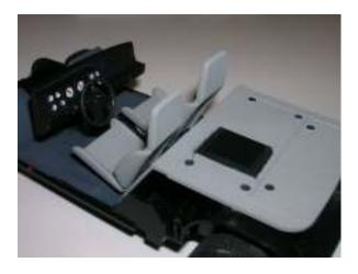
The dashboard was painted black and the instrument detail was painted with a brush. The floor shifter completed the interior.
