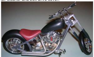
The design is relatively simple, especially when compared to the Tamiya 1/12 bike kits. But then it is about a third the cost. The tube frame is two main pieces. It fits together well, but in order to secure the front fork, the fork mount on the front of the frame clamps around the fork, which means there is a seam that needs filling once the pieces are assembled. Also, the frame cannot GTR Auto Modelers Newsletter
