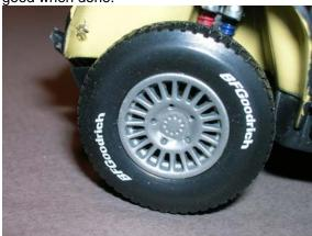
The wheels come pre painted silver, the tires are rubber vinyl with the Goodrich logos applied, and these mount onto metal axles. The chassis is one basic piece, with molded in suspension arms. There are separate shock absorber pieces that snap in, while these come painted I did some touch ups because the visible edges were not fully covered..
